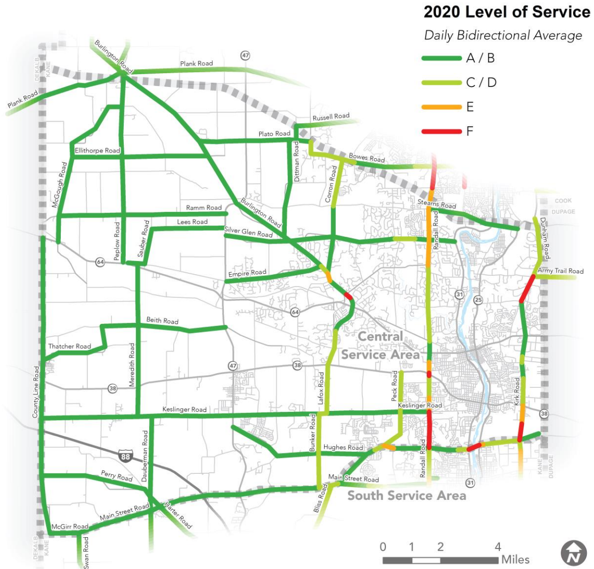
FIGURE 1-4: MODELED 2020 LEVEL OF SERVICE, CENTRAL SERVICE AREA
